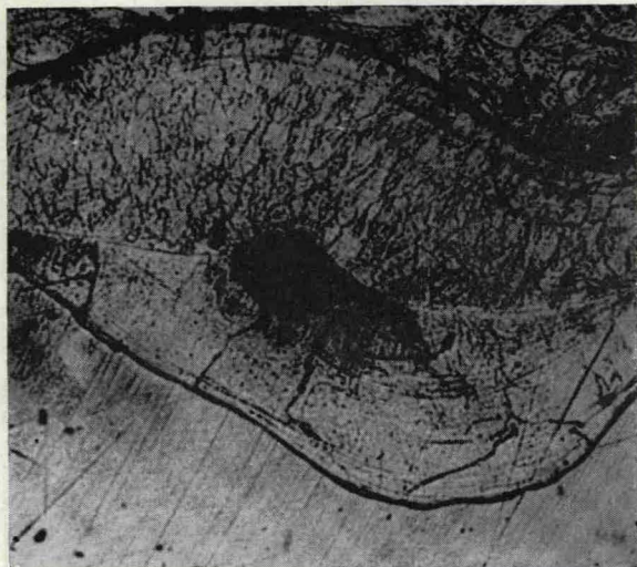
53 Solidification cavity in copper-to-nickel bond. \times 280 . [Courtesy Weld. Research Council. (Holtzman and Cowan. 21 )
