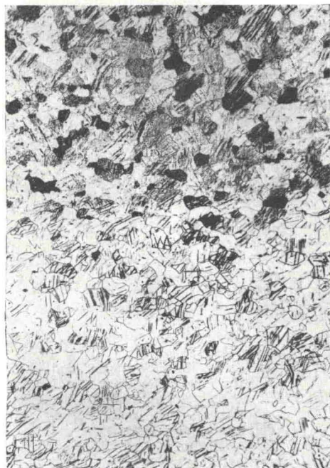
59 Shocked zone in iron. \times 80 .
