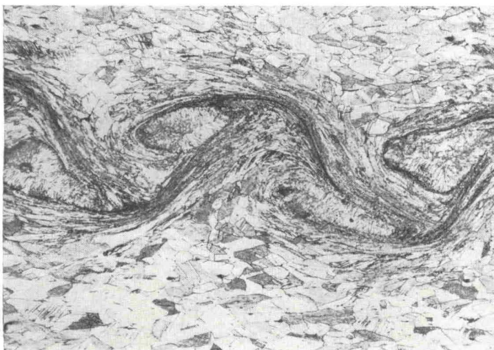
15 Wavy interface with fusion pockets produced by small angle of incidence and excessive charge. \times 100 .
