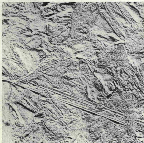
54 Carbon replica of vortex of a weld in low-carbon steel. \times 850 .
