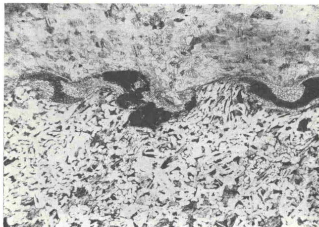
19 Micrograph of a steel weld made by using a knurled base plate. \times 45 .
